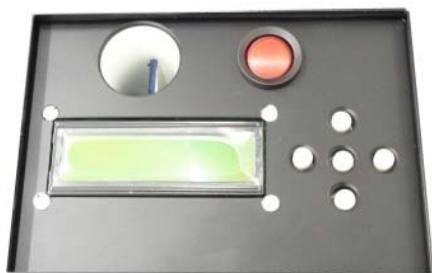
Control unit with backlight LCD screen and 5 control buttons.
